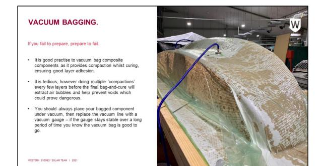
Once the layup schedule has been complete, It's time to 'bag' the part. The term 'Bagging' is jargon and describes the process in which the composite part is sealed and placed under a vacuum to cure, ensuring good layer adhesion and accurate tolerance.
