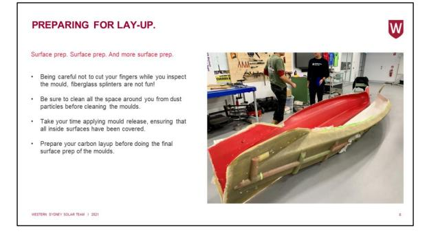
Once the mould cures, it needs to be pried off the buck. There are a variety of tools to use including PTFE wedges and air powered blasters. As you pull the mould off, you are able to see if there was any sticking thanks to that red or any bright coloured pigment used with the gelcoat.
