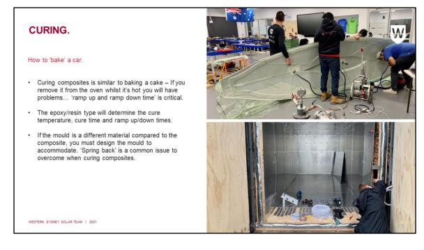
Whilst under vacuum, our prepreg composite parts need to be cured inside an oven, at temperatures ranging from 80 degrees celsius to 120 degrees celsius. An important thing to remember is ramp up and ramp down times - this refers to how quickly the temperature increases or decreases to ambient temperature. For our type of prepreg, this is usually around 1-2 degrees celsius per minute.
